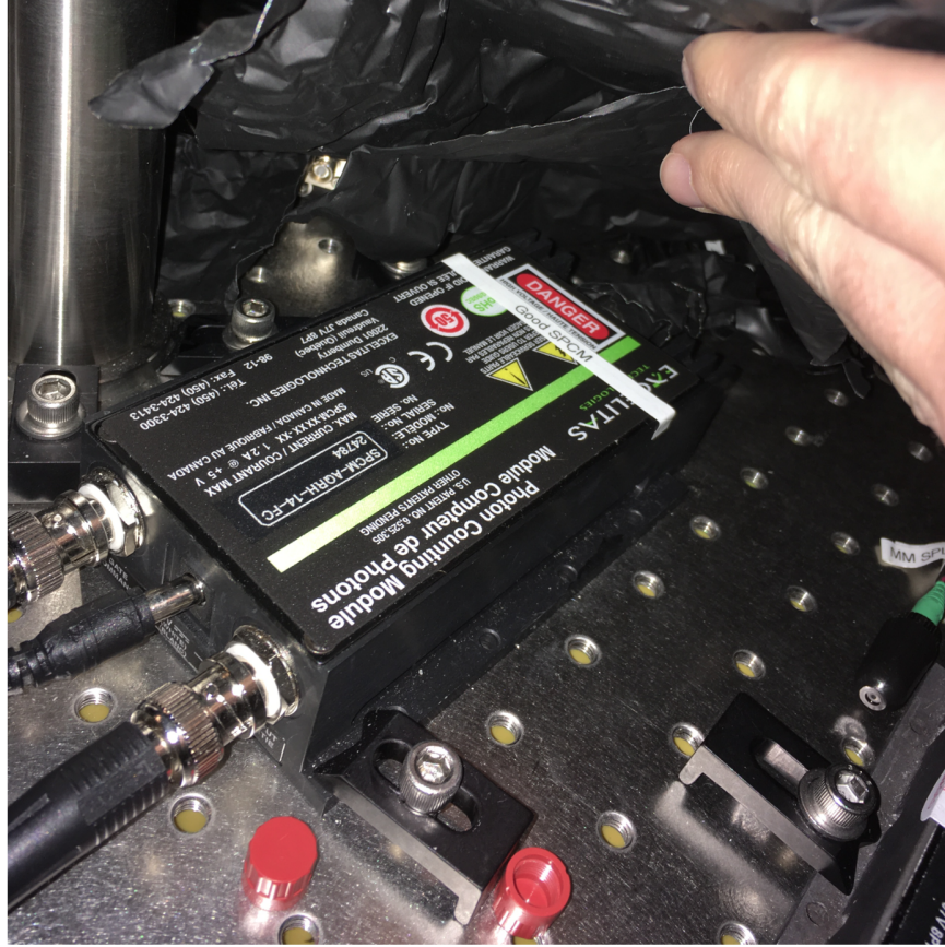
Figure 4.12: Single photon counting modules. We keep our SPCMs buried under many layers of foil because they are very sensitive to light. Never expose a powered-on SPCM to room light—it will get toasted! Always power off SPCMs in the event you think they will be exposed to light above their specified acceptable count rates.
